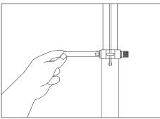
lock lever outward to loosen the clamp. not move, tighten the set screw into the Slide the handle up to desired height and handle. press the lever back inward to tighten.
