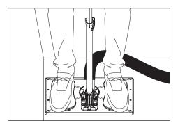
**4.** Place the SOS PRO in a starting point, usually a corner in the room and stand on it for about 5-30 seconds to extract water from the carpet and pad.
