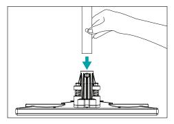
handle into the handle base. Make sure the spring button lines up with the hole. It will snap into place.
