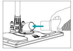
**1.** Connect vacuum hose from a portable **2.** Turn the extractor ON. or truck-mounted extractor. 2" cuffs will slide over the vacuum port and 1.5" cuffs will slide inside.
