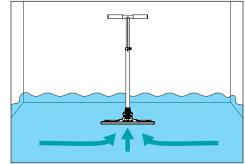
**3.** If there is standing water, place the SOS PRO in the center of the room to remove the standing water down to the carpet level.
