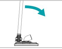
**5.** When you're ready to move to a new position, pull the handle back to release suction. Move the SOS PRO to a position that is directly adjacent to, but not overlapping, the previous extraction position.
